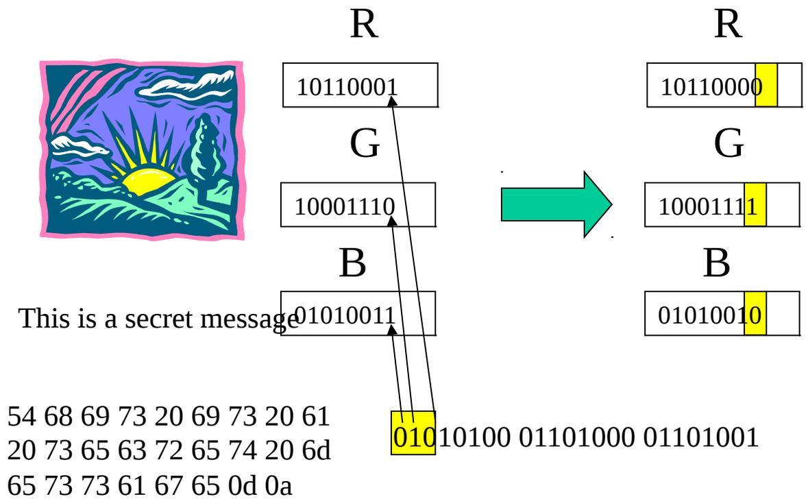
Least Significant Bit encoding hides a message in the LSB of an image. The image needs to have a certain variability. Additionally, the message can be encrypted. Changes in the LSB of a true color image are not noticeable for the human eye. But computers can detect „unusual“ bit frequencies
