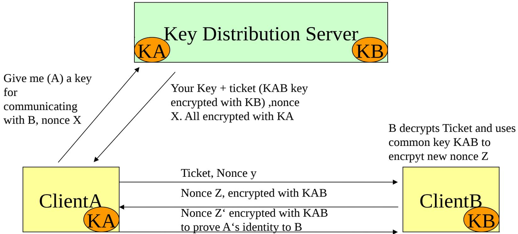
This protocol is used e.g. in Microsoft's Kerberos implementation. It requires a secure authentication server which knows the symmetric keys of all principals. A nonce is a request counter that is used to fend off replay attacks. A ticket contains a common key ( $K_{AB}$ ) and a partner name, both encrypted with the receivers secret key. Note that the secret keys of A or B (or passwords) do NOT go over the wire
