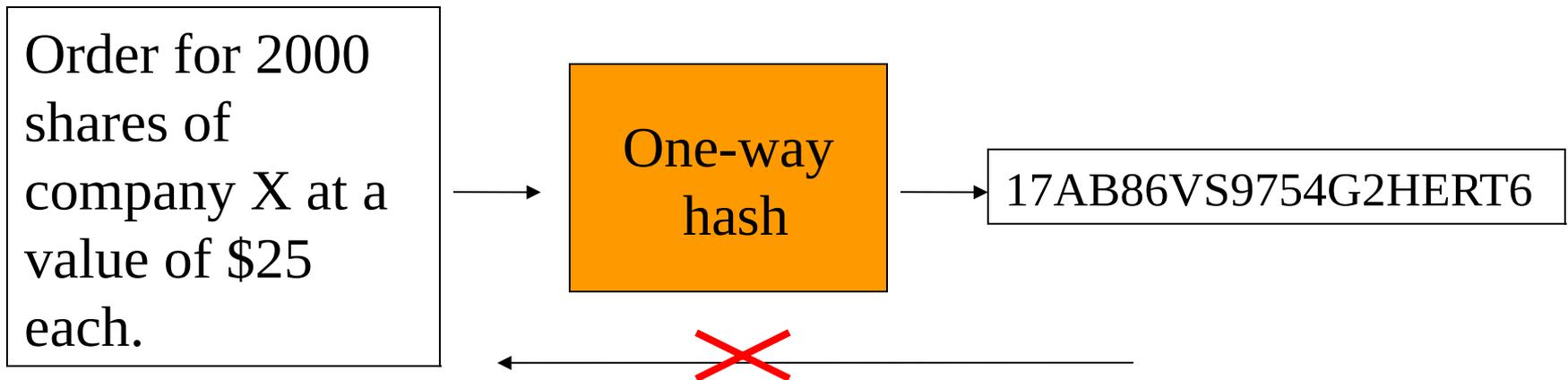
A one way hash function creates a fixed length representation of the input (with padding if necessary). The function guarantees that it is computationally infeasible to reverse the process and that no two different inputs will create the same output. A change in the input will cause a completely different output. This can be used to detect TAMPERING during message transfer. Popular one-way hash algorithms are Message Digest 5 (MD5) and Secure Hash Algorithm 1 (SHA1)
