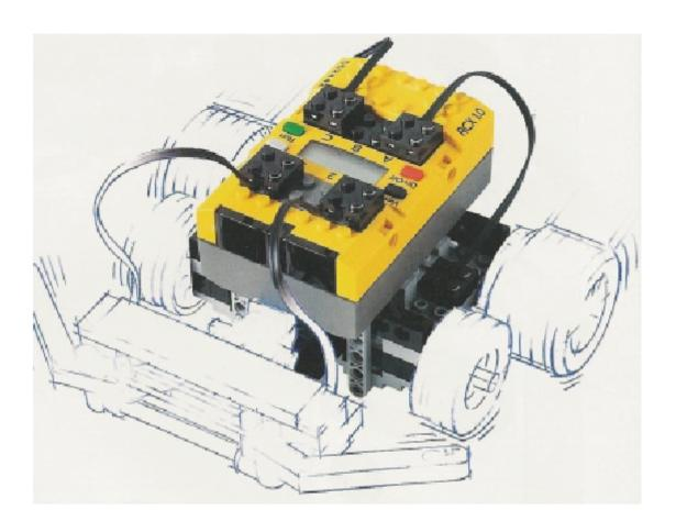
The Lego Mindstorms robot package is an example of a small embedded control platform. Several operating systems exist for this device, e.g. LegOS (c++) and Lejos (Java). A small Hitachi microprocessor and 32k of ram are available. We will use it as an example for embedded control programming (Using cross-compilation, firmware download and subsumption architecture). See http://www.jugs.org/protokolle/02-09-12/leJOS-v1.1.pdf
