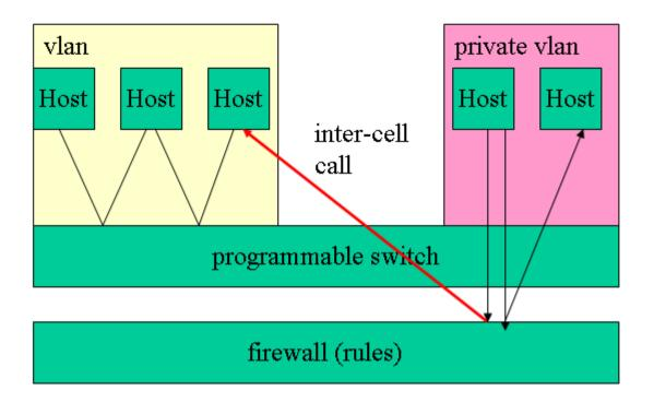
Based on private virtual lans, intelligent switches and network security cells a large scale firewall is designed to fit an international company. The vlan becomes "private" by routing all requests through the firewall – cell internal ones as well as cross cell requests. Several firewalls have been collapsed into one to ensure rule consistency.
