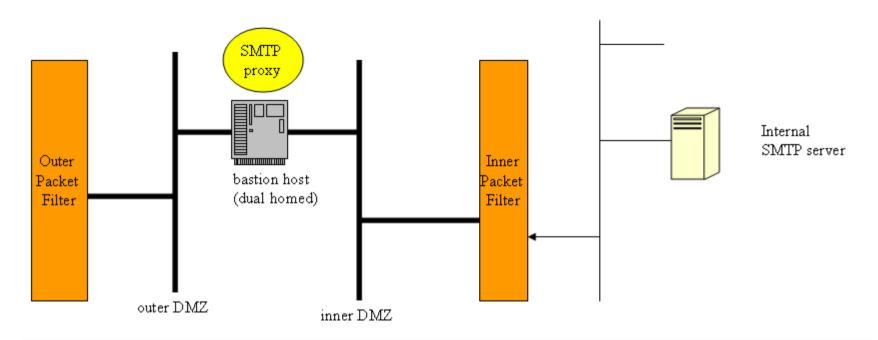
This configuration ensures that a) internal mail does not leave the intranet, b) all clients need to use the internal server which we can use for filtering/auditing etc. c) the connection to the outside will be configured correctly. The SMTP proxy on the bastion host will forward mails from outside to our internal mail server. Outgoing mail will be sent directly from the proxy on the bastion host to the destinations.
