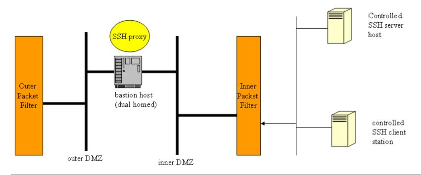
Because of the dangerous port forwarding feature outgoing SSH connections will only be allowed from controlled client stations (clients cannot install their own SSH clients wich might have port forwarding enabled). Incoming SSH will only be allowed (if at all) to a small number of controlled servers. Client and server authentication will use RSA public keys.
